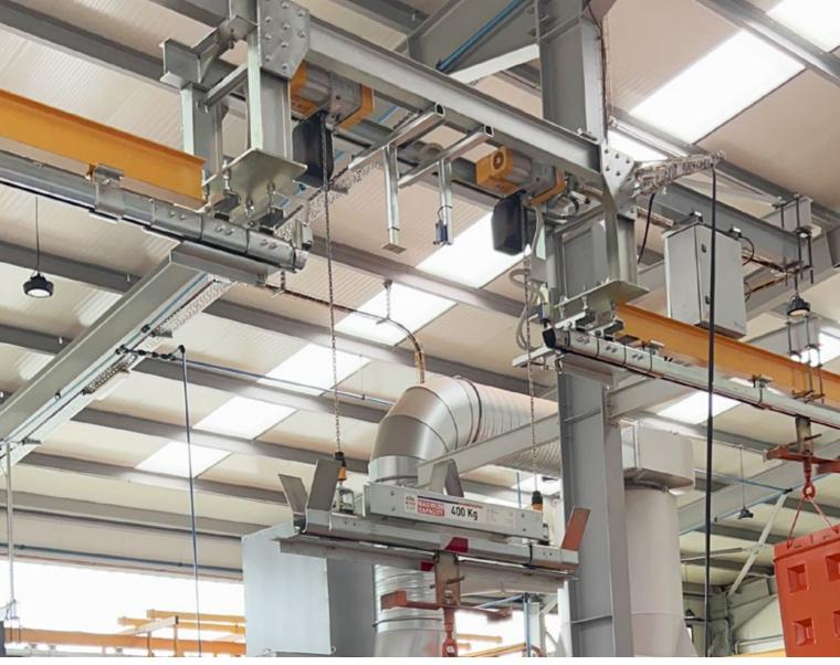
This system utilises a manual conveyor system and powers it through ovens, spray booths or any area where manual operation is not practical.
